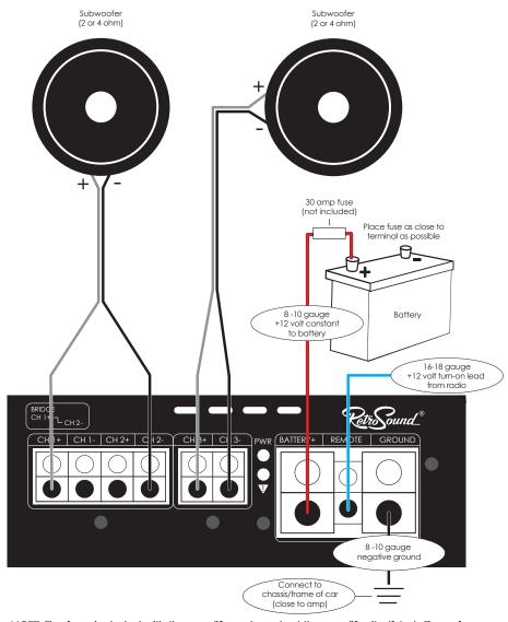
NOTE: The fuses included with the amplifier only protect the amplifier itself. Installing a fuse near the battery is required to protect your vehicle and wiring in case of a short-circuit. Check the fuse on the bottom of the amplifier for troubleshooting (30 amp ATC style).
