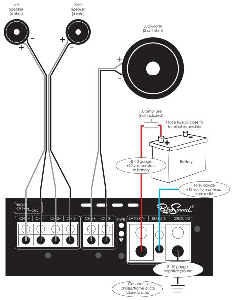
NOTE: The fuses included with the amplifier only protect the amplifier itself. Installing a fuse near the battery is required to protect your vehicle and wiring in case of a short-circuit. Check the fuse on the bottom of the amplifier for troubleshooting (30 amp ATC style).
